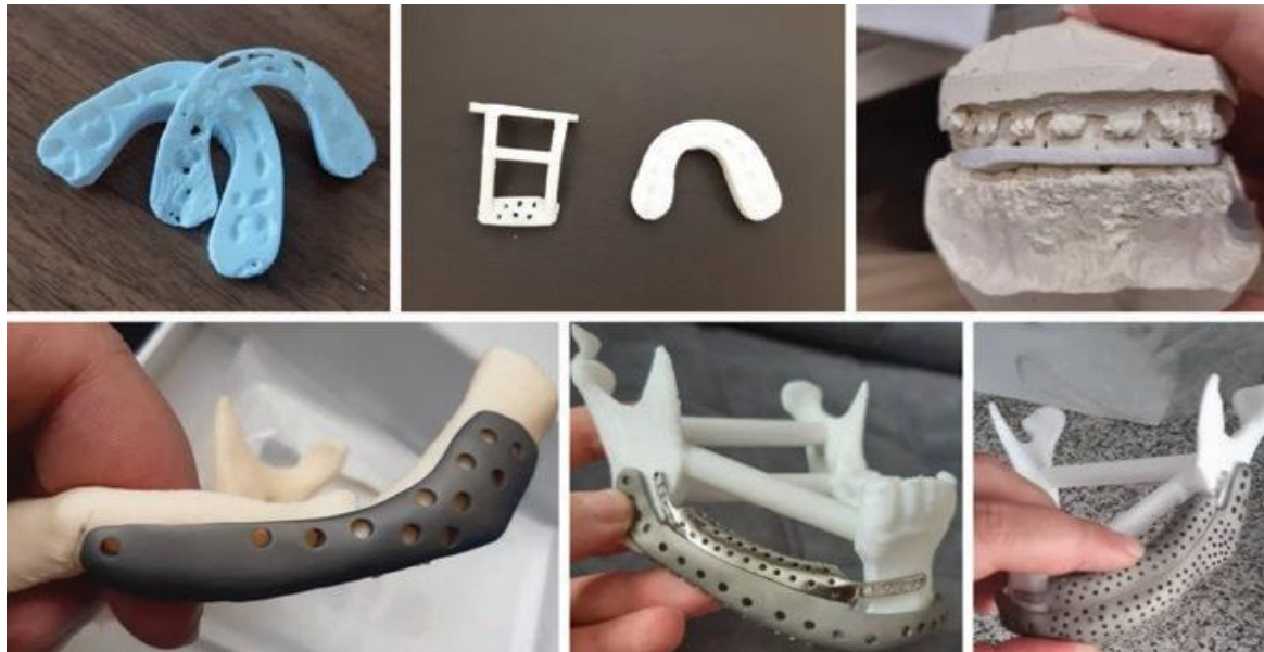
Fig. 6: Various 3D printed models using different additive manufacturing materials and printers. (a–c) Intermediate and final splint in orthognathic surgery, (d–f) mandibular titanium prosthesis for reconstruction of bony defects (23).
