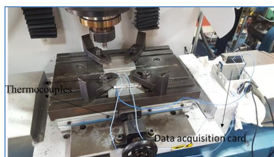
Fig.7: Connection for temperature measurement
