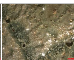
Fig.3 Phenomenon of celadon glazing shrinkage
